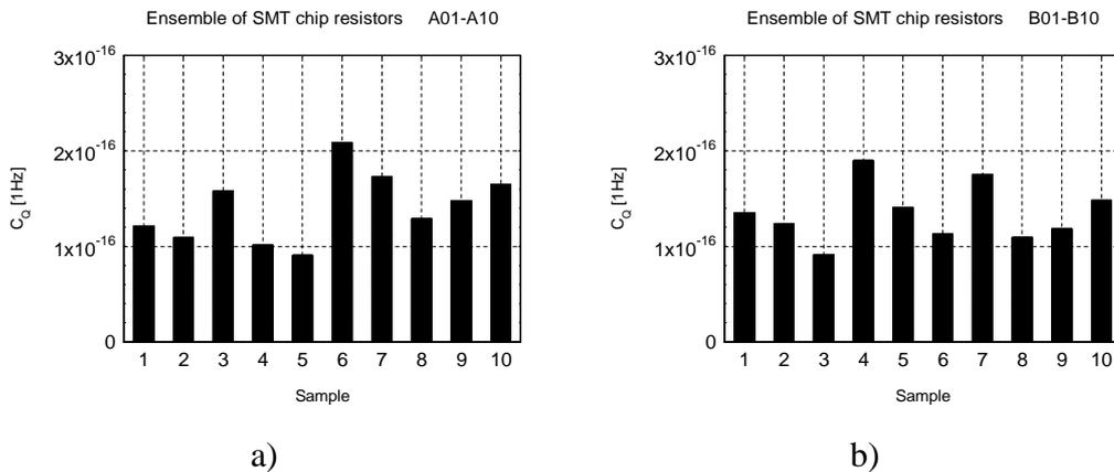
**Fig. 4:** The normalized noise voltage spectral density at 1Hz of samples
