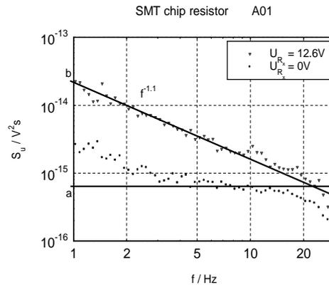
**Fig. 3:** The voltage noise spectral density of SMT chip resistor sample A01
