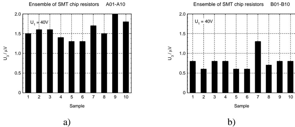
**Fig. 5:** Non-linearity measurement of samples a) A01 to A10, b) B01 to B10
