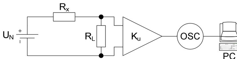
**Fig. 2:** Schematic chart of the noise experimental set-up
